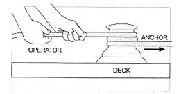
When recovering your anchor, first start the engine. In strong winds, tides, currents or in deep water, use a little engine power to come up over the anchor as the capstan is used. Never stall the capstan and do not run it at low speed for any extended time. Use one continuous and smooth recovery and do not repeatedly start/stop. If the anchor is stuck, use a little engine power and the weight of the boat to break it free.
